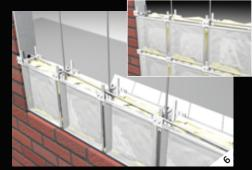
Lay half the quantity of mortar and fix the horizontal rod in position, not forgetting to put silicone in the holes, and then cover over the rod with remainder of mortar. Rods have to be positioned every row vertically and horizontally.
