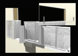
Note: Easifix spacer must always separate blocks from frame. Remember each row has to be secured with anchor brackets.
