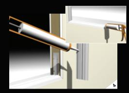
Take a 185mm length of spacer profile and silicon two beads of Easifix adhesive on one side. Place over the anchor bracket. Silicon two beads of Easifix adhesive to the Easifix spacer profile.
