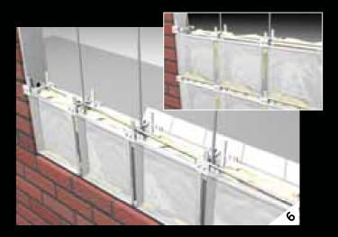
Lay half the quantity of mortar and fix the horizontal rod in position, not forgetting to put silicone in the holes, and then cover over the rod with remainder of mortar. Rods have to be positioned every row vertically and horizontally.
